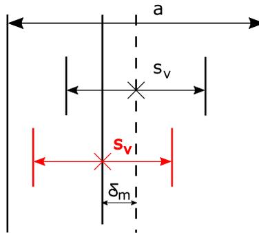
Figure 1: Errors in HD maps:  $a$ ... lane width,  $s_v$ ... car width,  $\delta_m$ ... HD map error
