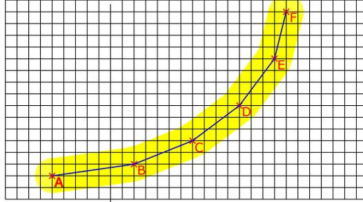
Figure 4: Trajectory: a curve approximated by line segments; the yellow area corresponds to the trace left by the moving disc
